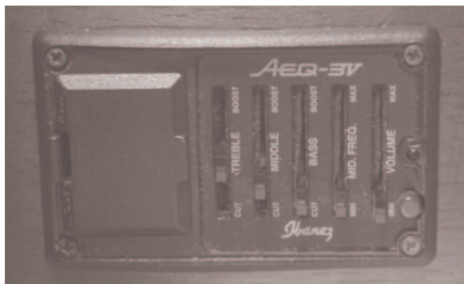
Figure 6.96 Built-in preamplifiers of acoustic guitars are often quite versatile. For example, Ibanez AEQ-3V is equipped with shelving graphic EQ for bass and treble plus a parametric control for mid-ranges. Tone-shaping capabilities of this preamplifier are far better than what the majority of guitar amplifiers can offer.
