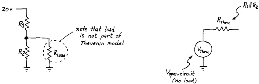
Figure N1.12: Thevenin Model: perfect voltage source in series with output resistance
