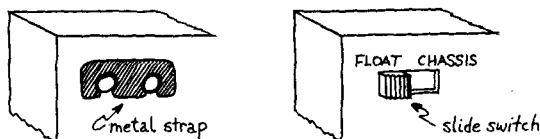
Figure L6.2: “Float” One Function Generator
