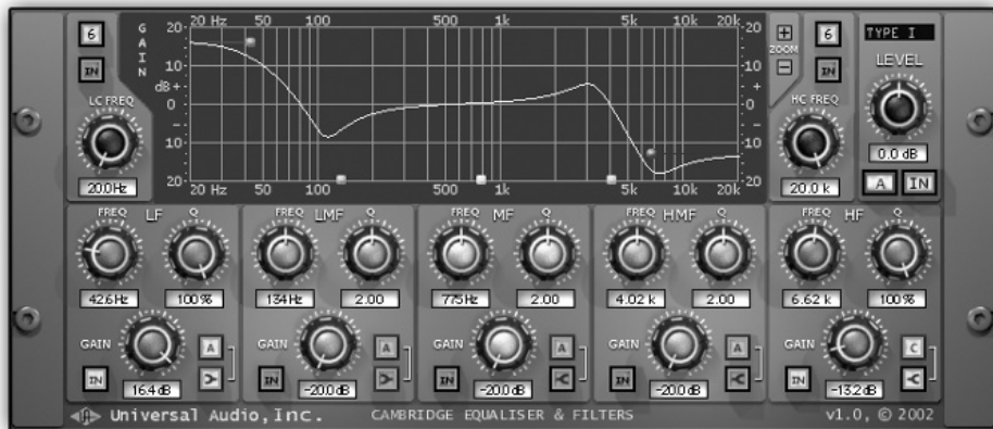
Figure 14.15 A typical contrast resonance on a shelving filter (the Universal Audio Cambridge EQ ). Both the low- and high-shelving filters are engaged in this screenshot, and it might be easier to discern them if we imagine a cross-line at 700 Hz. The low-shelving filter, set to type A, has a single contrast bend around the transition frequency. The high-shelving filter, set to type C, has two of these bends – one around the transition frequency, the other around the corner frequency.
