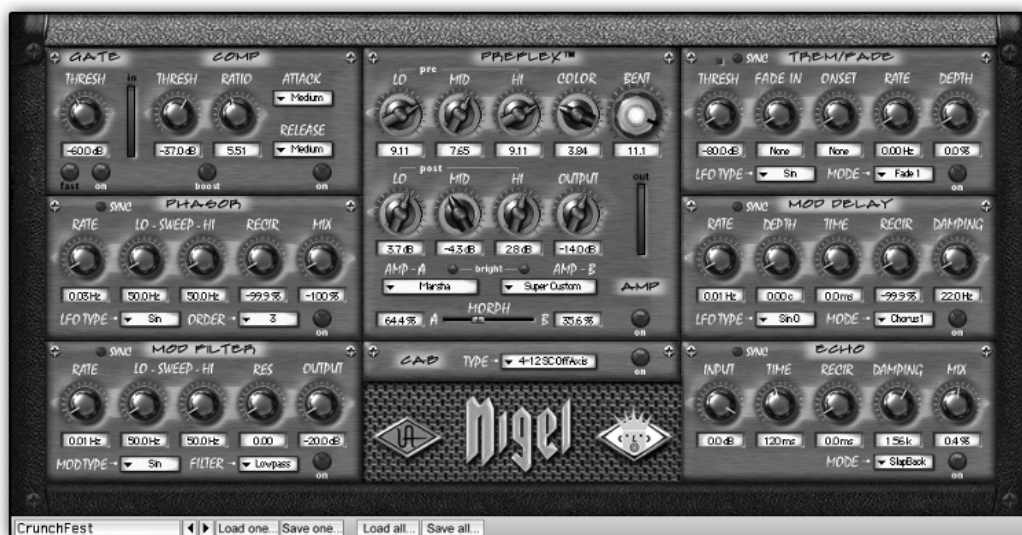
Figure 24.4 The Universal Audio Nigel . The center blocks on this plugin are the amp simulator where different amps and cabinets can be chosen. The side blocks provide additional effects like tremolo and delay.
