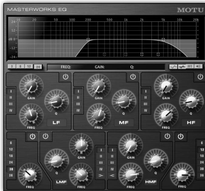
Figure 14.31 A HPF and LPF combined to form a band-pass response (the MOTU Masterworks EQ ). The two filters are set to remove frequencies below 200 Hz (HPF) and above 5 kHz (LPF). Band-limiting instruments in a similar way can increase separation and reduce masking.
