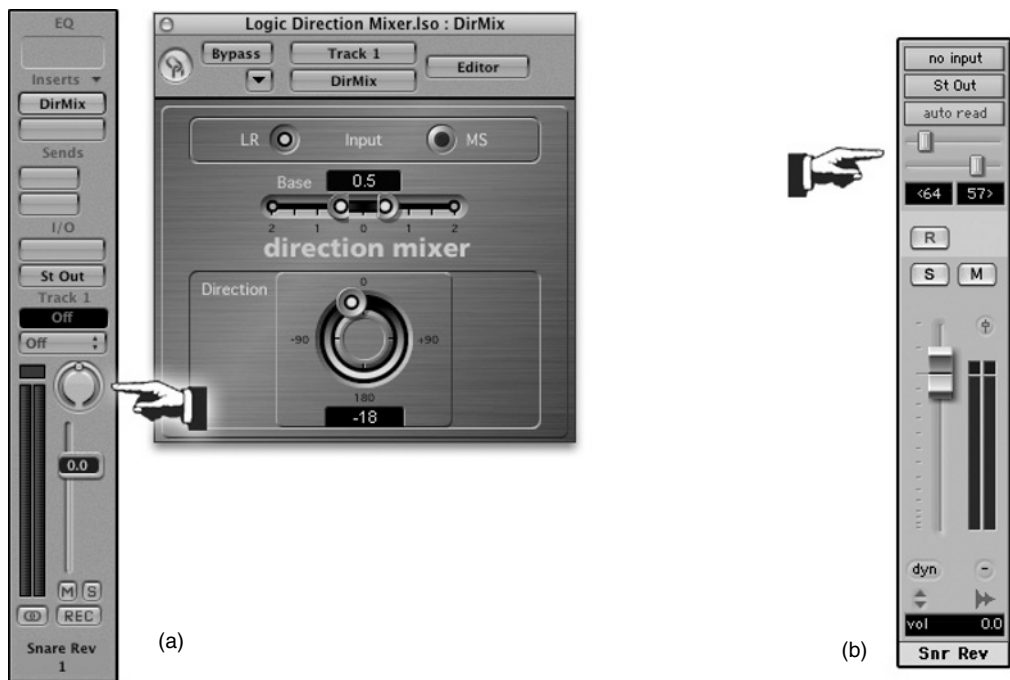
Figure 13.14 (a) Logic only offers balance control for stereo tracks. More control over stereo image can be achieved with the help of the direction mixer plugin. (b) Pro Tools offers dual-mono pan control for stereo tracks, which provides full functionality for any stereo imaging task.
