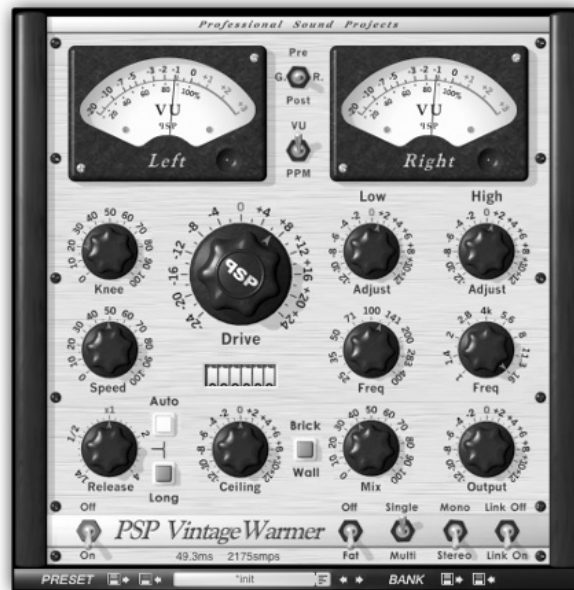
Figure 16.41 The PSP VintageWarmer 2 . The Mix control (to the right of the Brick Wall switch) lets us blend the unprocessed input with the compressed version, making parallel compression a very easy affair.
