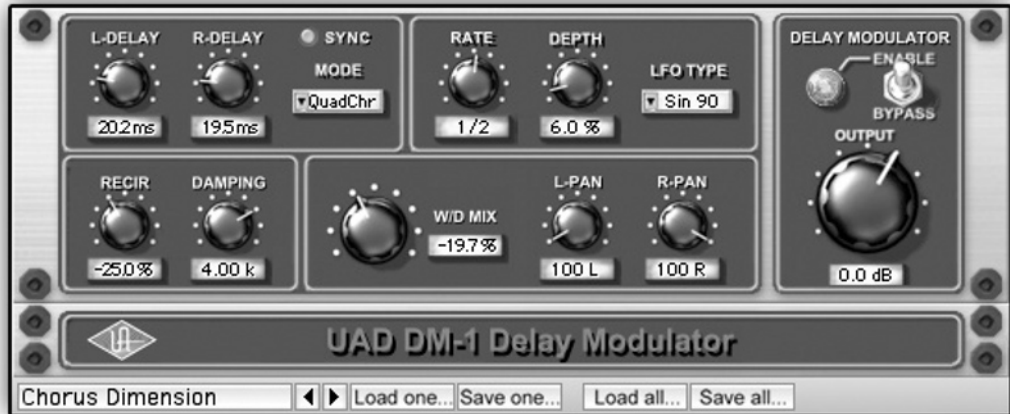
Figure 22.1 The Universal Audio DM-1 in chorus mode. This screenshot shows the settings of the Chorus Dimension preset. Essentially, very short delay on both channels, negative feedback of 25% and feedback filter set to 4 kHz; slow rate, little depth and only 19.7% of wet signal which is phase inverted.
