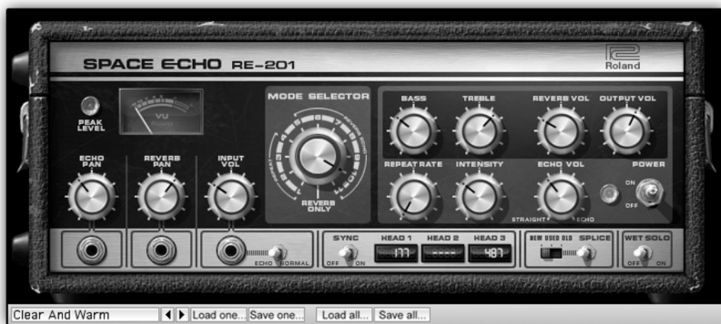
Figure 21.1 The Universal Audio Roland RE-201 Space Echo . This plugin for the UAD platform emulates the sound of the vintage tape loop machine. The interface looks very similar to that of the original unit.
