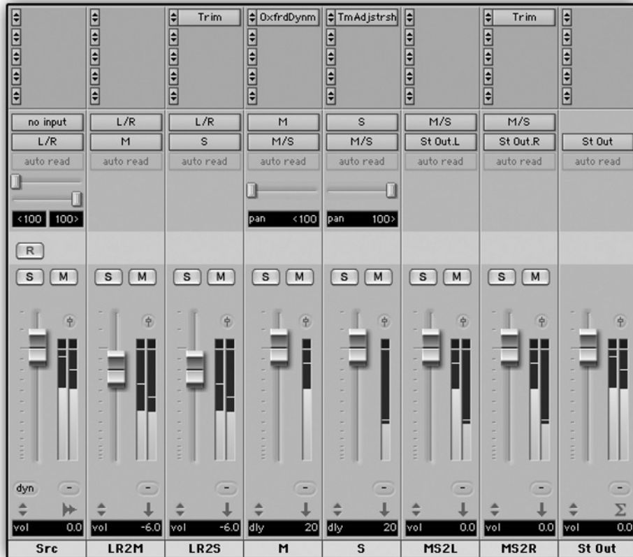
Figure 26.2 LR and MS conversion in Pro Tools. The original track is routed to the L/R bus, which feeds both the LR2M and LR2S auxiliaries. Since the output of LR2M is mono, the left and right channels are summed. There is also 6 dB attenuation corresponding to the required halving. LR2S does exactly the same, only that using the Trim plugin the right channel is phase inverted, resulting in mono output which is the difference between left and right (attenuated by 6 dB). The M and S buses are each fed into a mono auxiliary, where each can be processed individually. The Time Adjuster plugin was only inserted on S to manually compensate for the 20 samples plugin delay the Sonnox Oxford on M involves. Both M and S are panned to the extremes and routed to a different bus called M/S, which feeds both the MS2L and MS2R auxiliaries. These two auxiliaries feed the respective left and right channels of the St Out bus. While MS2L simply sum M and S, the Trim plugin on MS2R inverts the phase of S, thus the mono output is the difference between M and S.
