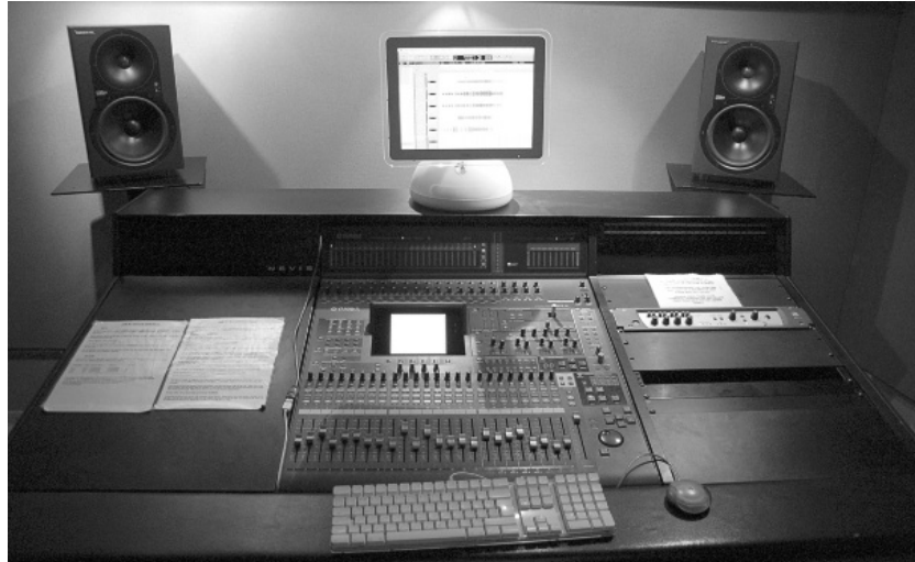
Figure 9.35 The Yamaha O2R96 studio at SAE Institute, London. This desk provides 4 layers, each consisting of 24 channels (or buses). Had this desk's layers been unfolded, it would be fourfold in size. The monitors in this photo are the Mackie HR824s.
