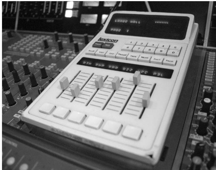
Figure 23.4 The ‘larc’ (remote control) for the Lexicon 480L; the reverb unit itself is rack-mounted and often unseen in studios. Despite being released in 1986, the 480L is still considered by many as one of the best reverb emulators (courtesy of SAE Institute, London).
