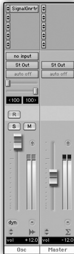
Figure 10.10 This Pro Tools screenshot shows a signal first being boosted by 12 dB by the audio track fader, then attenuated by the same amount using the master fader. Despite the lit clipping indicator on the audio track, this setup will not generate any clipping distortion.
