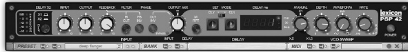
Figure 22.3 The PSP Lexicon 42 in deep flanger mode. This screenshot shows the setting of the deep flanger preset – high feedback, 1 ms of delay, high depth, slow rate and both the feedback signal and the wet signal are phase inverted.
