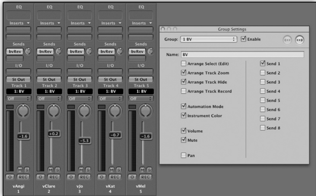
Figure 10.4 Logic’s control grouping. The various backing-vocal tracks all belong to control group 1 – titled BV. The linked properties are ticked on the group settings window.
