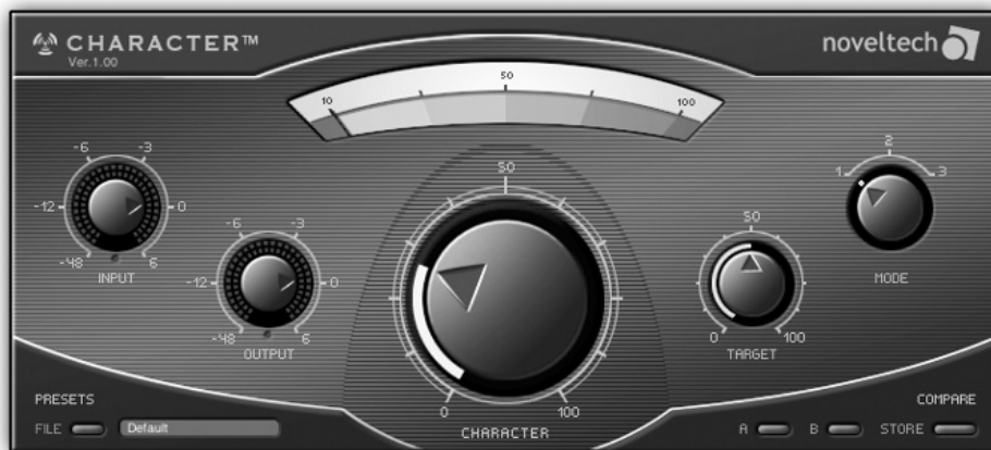
Figure 26.4 The Noveltech Character plugin. The enhancement process is granted by three mere controls: character, target and one of three modes.
