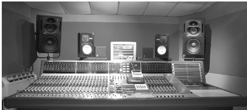
Figure 7.3 The NEVE VRL studio at SAE Institute, London. The three sets of monitors can be seen here: the full-range are the Genelec 1037Bs, the near-fields are the NS10s and the mini-speakers are the AKG LSM50s.
