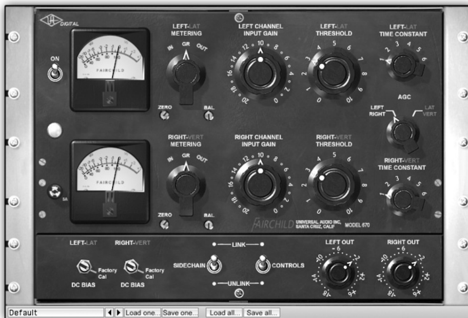
Figure 26.1 The Universal Audio Fairchild plugin. This plugin looks and works very similar to the original unit (the price of which can easily exceed the $25 000 mark on the vintage market). Like the original unit, the plugin can work in either left/right or mid/side modes (determined by the control between the two channels). The mid/side mode is labeled Lat/Vert (lateral/vertical) as per the stereo record cutting method.
