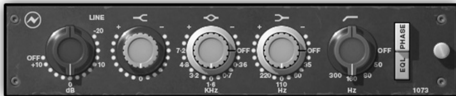
Figure 14.11 The Universal Audio NEVE 1073 EQ plugin. This plugin, which emulates the sound of the analog legendary NEVE 1073 , has a frequency response which deviates from the perfect theoretical shape of filters, a fact that contributes to its appealing sound. The high-pass filter (rightmost control) involves changing resonance for each of the four selectable cut-off frequencies.
