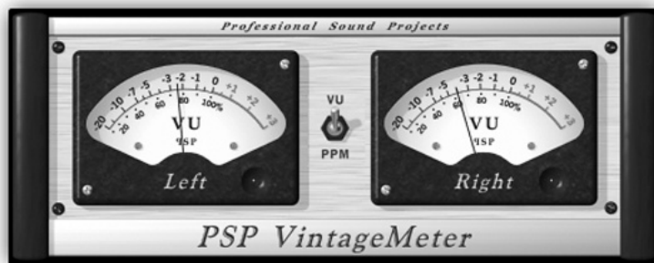
Figure 8.4 The PSP VintageMeter . This free plugin offers averaging metering characteristics similar to those on the mechanical VU meters.
