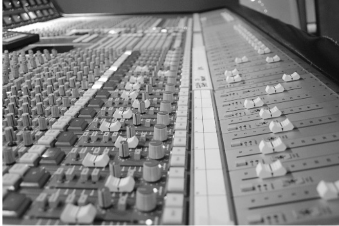
Figure 9.21 The SSL 4000 G+. This photo clearly shows the two faders per I/O module. Depending on the desk configuration, one fader controls the level of the monitor path, the other the channel path (courtesy of SAE Institute, London).
