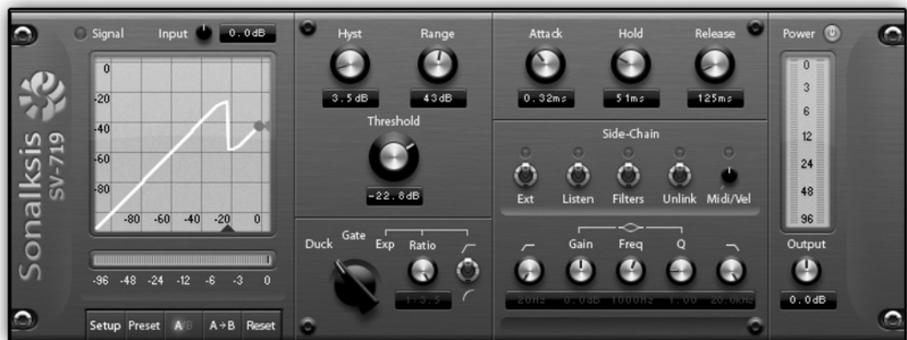
Figure 20.1 The Sonalksis SV-719 . This gate/expander plugin also offers a ducker mode.
