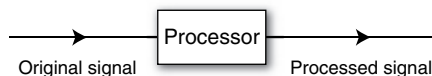
Figure 9.1 Processors are connected in series to the signal path and replace the original signal with the processed one.
