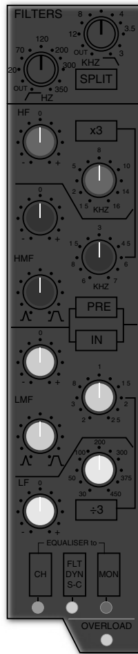
Figure 14.5 A diagram of the SSL 4000G+ equalizer. The equalizer section consists of four bands: the LF and HF bands are shelving filters, the LMF and HMF are parametric equalizers. At the top: a high- and low-pass filters.
