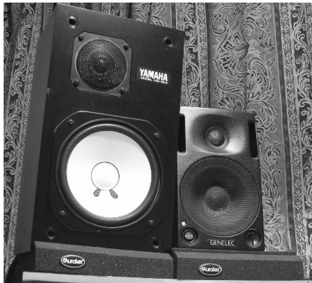
Figure 7.5 The Auralex MoPAD monitor isolation pads. Both a Yamaha NS10 and a Genelec 1029 are shown here resting on the Auralex MoPADs.
