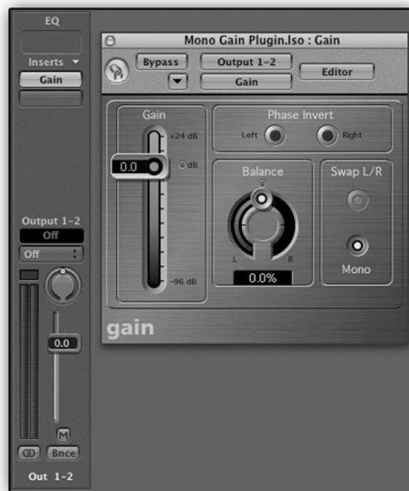
Figure 5.1 Logic's Gain plugin enables summing a stereo signal to mono.
