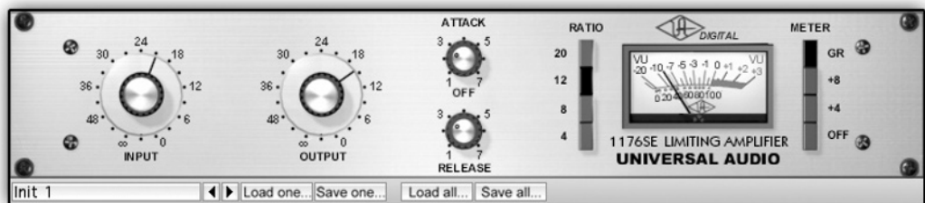
Figure 16.7 The Universal Audio 1176SE . This plugin for the UAD platform emulates the legendary Urei 1176 LN. It has fixed threshold and the degree of compression is partly determined by the input gain amount.
