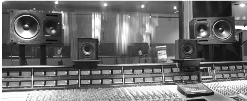
Figure 7.2 The Auratones 5C are the mini-speakers mounted on the meter bridge. Behind them are the Genelec 1031s near-fields (Courtesy of SAE Institute, London).
