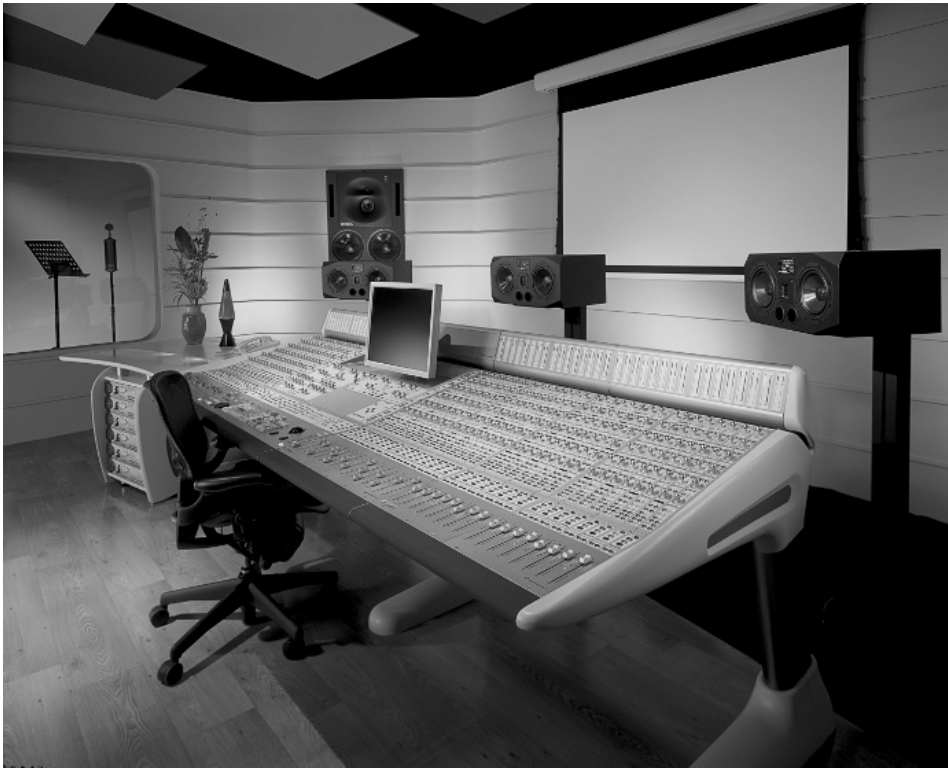
Figure 27.4 The Digidesign Icon D-Control . This product, which looks like a large-format console, is a pure control surface for Pro Tools. Products of this kind enable a mixing experience that was a reserved asset of large-format consoles, with all its technical and creative benefits (courtesy of Digidesign, Bill Schwob Photo).
