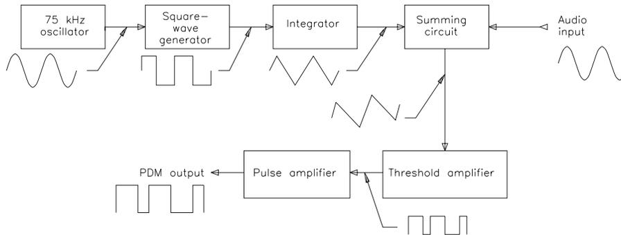
**Figure 5.9** Block diagram of a PDM waveform generator.
