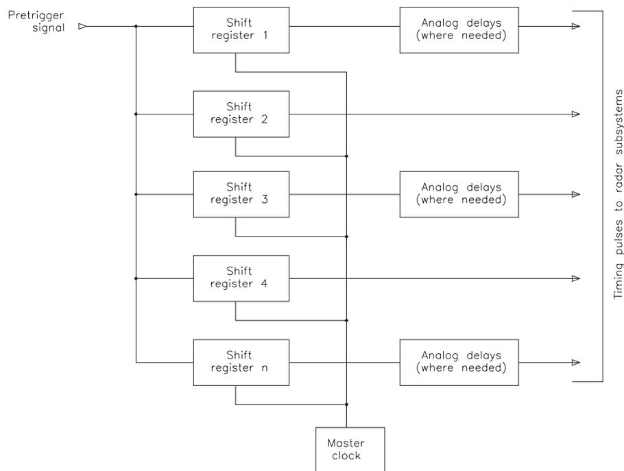
**Figure 5.26** Digital synchronizer system for radar applications.
