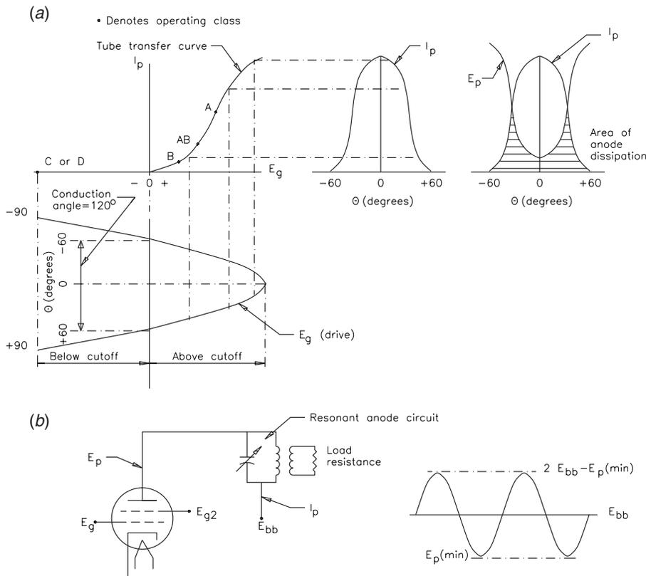
**Figure 5.5** Classic vacuum tube class C amplifier: (a) representative waveforms, (b) schematic diagram. Conditions are as follows: sinusoidal grid drive,  $120^\circ$  anode current, resonant anode load. (After [2].)
