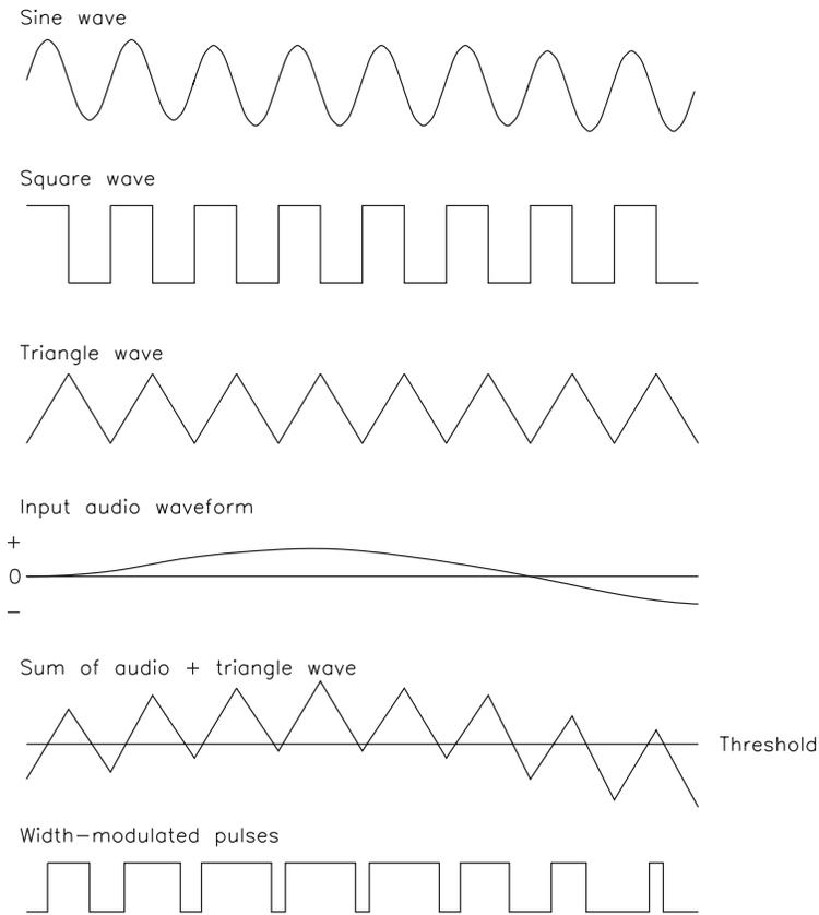
**Figure 5.8** The principal waveforms of the PDM system.
