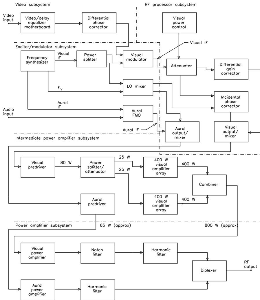
**Figure 5.18** Basic block diagram of a TV transmitter. The three major subassemblies are the exciter, IPA, and PA. The power supply provides operating voltages to all sections, and high voltage to the PA stage.
