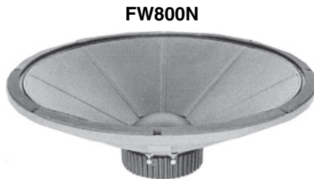
Figure 2.8 A very large loudspeaker – a 30 inch (800 mm) low frequency loudspeaker with radial reinforcing ribs to augment the cone rigidity
