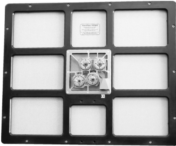
Figure 2.25 A distributed-mode loudspeaker (DML)
