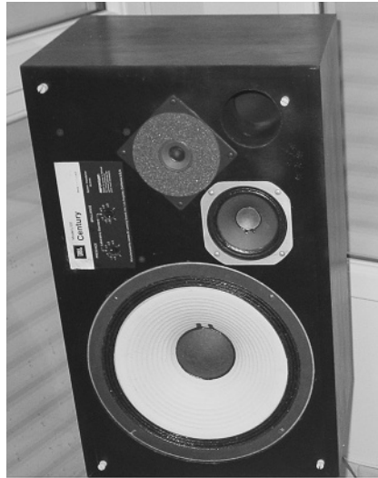
Figure 2.6 A full-range, all cone driver loudspeaker system – the JBL L100
