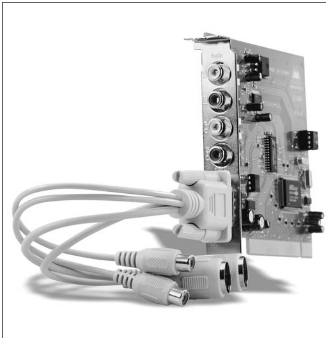
Figure 2-2: Some PCI interfaces often come with analog connectors run from the computer.
