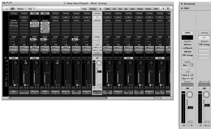
Figure 14-1: Left: The main mixer menu in a software mixer. Right: The channel strip section of the mixer.
