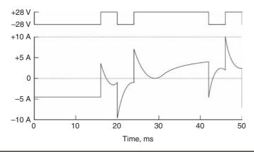
FIGURE 22.6 Peak loudspeaker currents with a special test signal.
