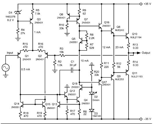
FIGURE 3.12 Amplifier with cascoded VAS.
