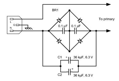
FIGURE 16.15 Keeping mains DC off the power transformer primary.
