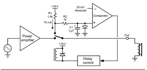
FIGURE 15.13 A simple load-sensing circuit.
