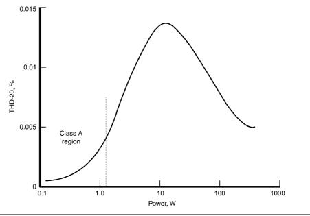
**FIGURE 3.15** THD-20 versus power into  $4-\Omega$  load.
