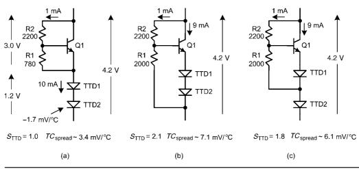
FIGURE 14.18 Three bias spreaders for ThermalTrak output transistors.
