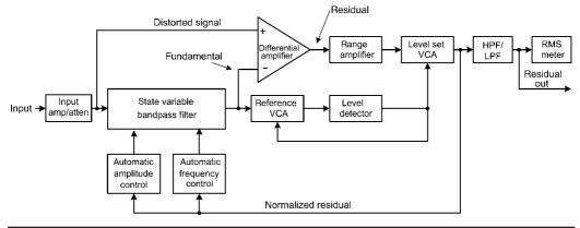
FIGURE 21.2 Block diagram of a typical THD analyzer.
