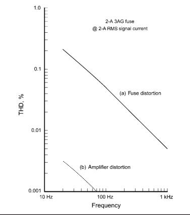
FIGURE 13.4 THD versus frequency for a 2-A fuse passing 2 A RMS.
