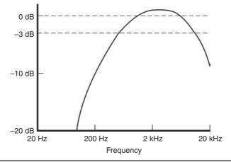
FIGURE 1.3 A weighting frequency response.
