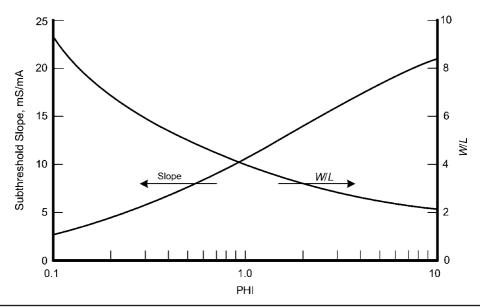
FIGURE 20.15 Subthreshold slope and desired value of W/L as a function of PHI.
