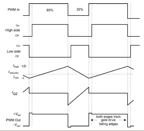
FIGURE 29.3 Current waveform of low side transistor Q2 when duty cycle is 65%.
