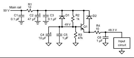
FIGURE 13.1 Filtering the power supply with a capacitance multiplier.
