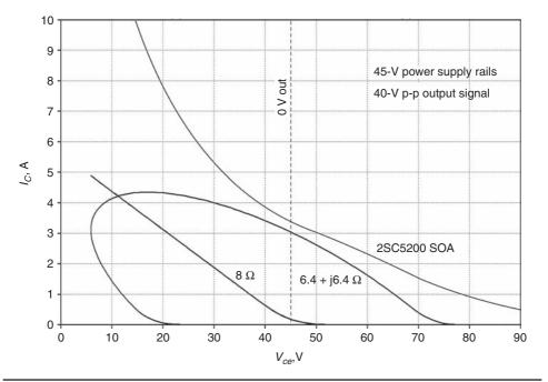
**FIGURE 15.4** Positive-current portion of the reactive load line plotted against  $V_{\infty}$ .
