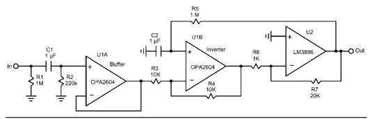
**FIGURE 27.2** Gain Clone in inverting mode reduces input common-mode distortion and eliminates the electrolytic capacitor.
