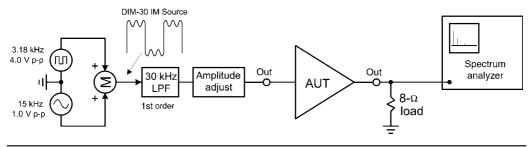
FIGURE 22.3 The DIM test for transient intermodulation distortion (TIM).
