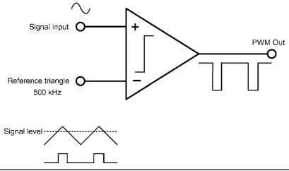
FIGURE 28.1 A simple PWM modulator.
