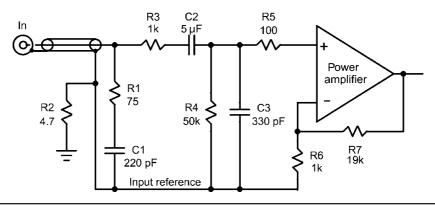
**FIGURE 18.5** Amplifier input circuit with a Zobel network.
