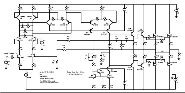
FIGURE 11.17 A high-performance MOSFET power amplifier.
