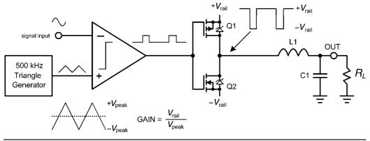
FIGURE 28.2 A simple PWM class D amplifier.
