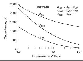
FIGURE 28.5 Capacitances for the IRFP240 N-channel MOSFET.
