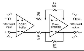
FIGURE 26.7 A true balanced amplifier with differential-mode feedback.
