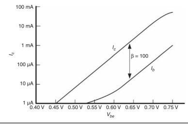
FIGURE 2.2 Transistor Gummel plot.
