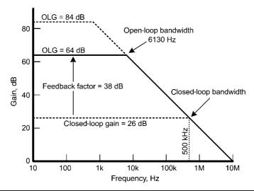
FIGURE 3.6 Reduced open-loop gain with degeneration.
