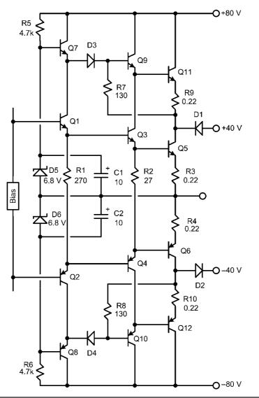
FIGURE 5.10 Class G output stage design.
