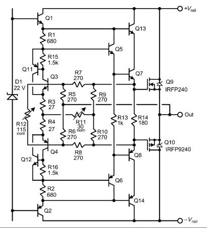
FIGURE 12.10 Use of a CFP-based error amplifier and cascoded drivers.
