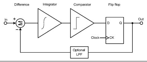
FIGURE 30.5 A simple analog sigma-delta modulator.
