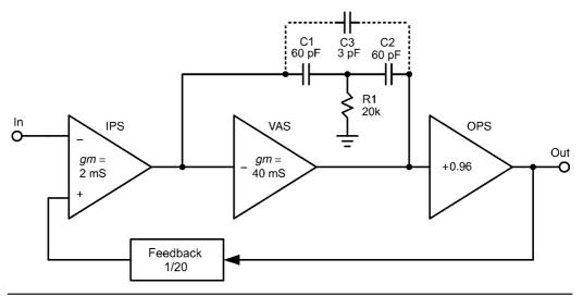
FIGURE 9.4 An amplifier with two-pole compensation.
