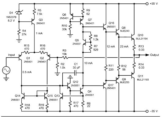
FIGURE 3.10 Output stage with Triple emitter follower.
