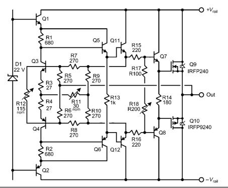
**FIGURE 12.8** An EC circuit suitable for use with low- $V_{es}$  MOSFETs.
