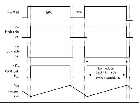
FIGURE 29.2 PWM waveforms when duty cycle is 75%.
