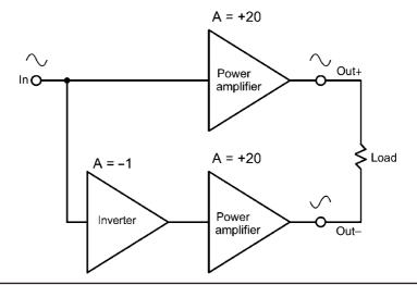
FIGURE 26.6 A bridged power amplifier.
