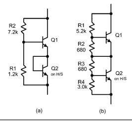
**FIGURE 11.8** Bias spreader  $V_{pe}$  multipliers for vertical MOSFET output stages.
