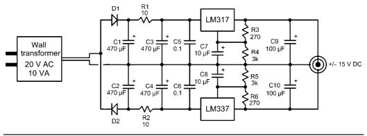
FIGURE 21.7 Wall transformer power supply for test gear.
