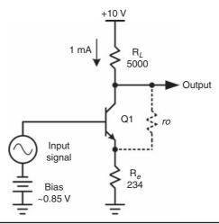
FIGURE 2.5b CE stage with emitter degeneration.
