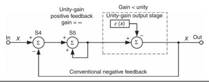
**FIGURE 12.3** HEC viewed as negative feedback whose open-loop gain is enhanced by an embedded positive feedback loop.
