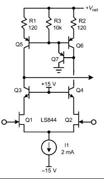
FIGURE 7.7 A cascoded JFET input stage.
