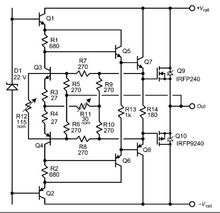
FIGURE 12.5 A simple error-correction circuit for a MOSFET output stage.
