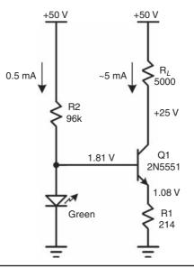
FIGURE 2.10c Current source using LED.
