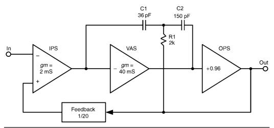
FIGURE 9.9 Amplifier with transitional Miller compensation.
