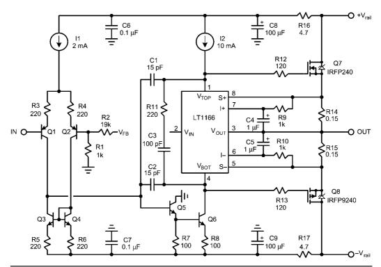
FIGURE 27.9 A simplified amplifier using the LT1166.
