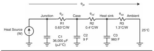
FIGURE 14.2 Thermal model for a power transistor mounted to a heat sink.
