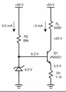
FIGURE 2.10d Current source using Zener diode.
