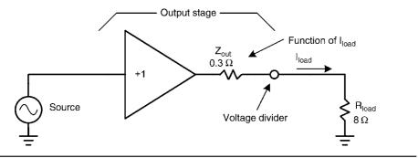
FIGURE 5.3 Amplifier output stage gain.
