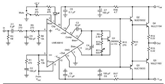
FIGURE 27.5 A simplified power amplifier based on the LME49810.
