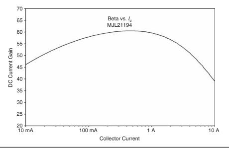
FIGURE 20.4 Current gain beta versus collector current.
