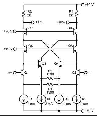
FIGURE 25.10 The Cascomp differential input stage.
