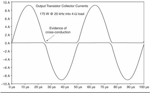
FIGURE 10.9 Output transistor current waveform.
