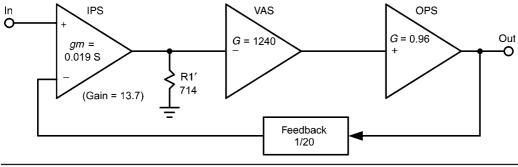
FIGURE 2.13 Amplifier gain at low frequencies.
