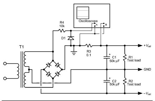
FIGURE 16.10 Measuring rectifier performance.
