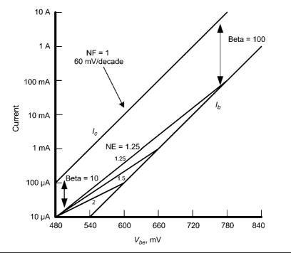
FIGURE 20.10 Effect of NE on beta versus I<sub>c</sub>.
