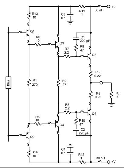
FIGURE 10.15 An output Triple with stray inductances shown.
