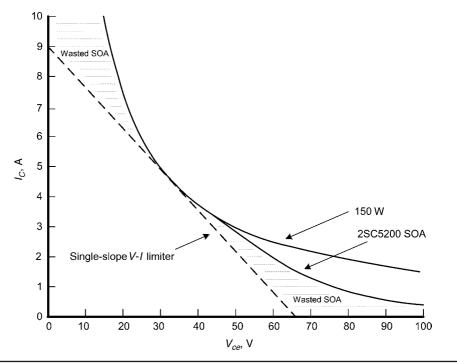
FIGURE 15.15 Single-slope V-I limiter action plotted with SOA curve.
