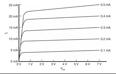
FIGURE 2.1 Transistor collector current characteristic.
