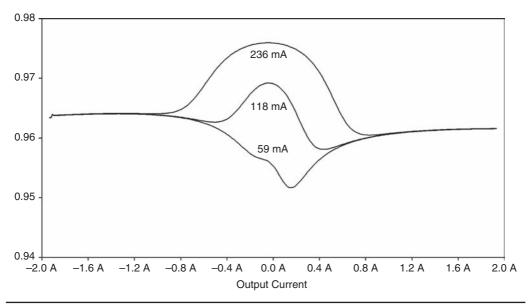
FIGURE 10.2 Wingspread plot illustrating the crossover distortion mechanism.
