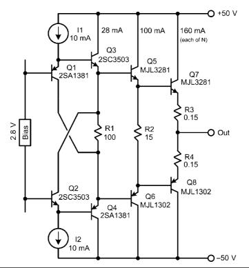
FIGURE 25.7 A BJT output Quad including a diamond buffer.
