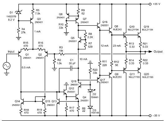
FIGURE 3.13 Amplifier with double output stage.
