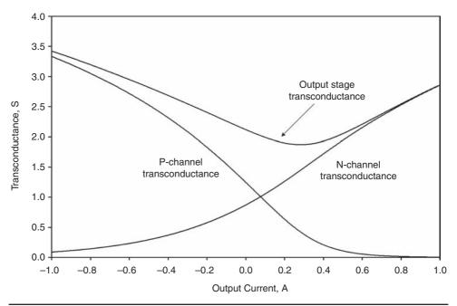
FIGURE 11.10 Illustration of transconductance droop for IRFP240/9240 output pair.
