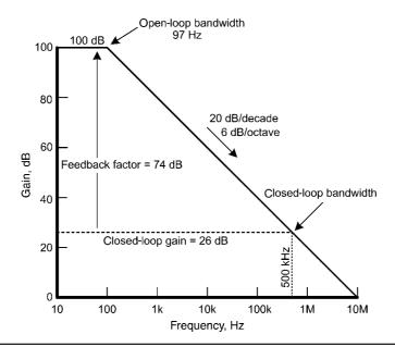
**FIGURE 3.9** Performance with IPS current mirror load.
