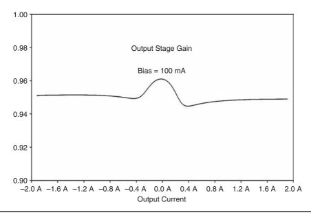
FIGURE 5.4 Output stage gain versus output current.
