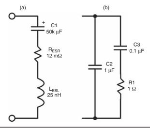
**Figure 16.7** (a) Simplified equivalent circuit for a 50,000-µF reservoir capacitor. (b) A bypass/ snubber arrangement.
