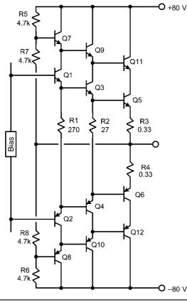
FIGURE 5.8 Stacked output stage design.
