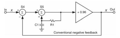
**FIGURE 12.4** Compensating the error-correction loop.
