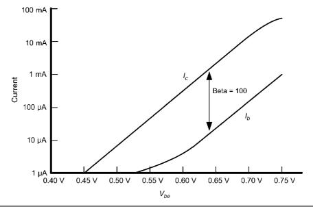
FIGURE 20.6 Transistor Gummel plot.
