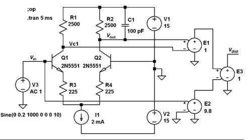
FIGURE 19.3 Simulation circuit for viewing input-output error.
