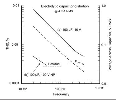
FIGURE 13.3 THD versus frequency for a 100-µF nonpolarized electrolytic capacitor.
