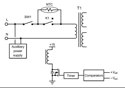
FIGURE 16.13 An active soft-start circuit.
