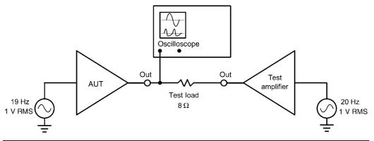
FIGURE 23.4 Two-tone back-feeding test using 19-Hz and 20-Hz test signals.
