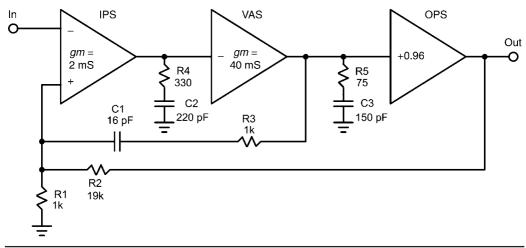
FIGURE 9.7 Amplifier with Miller input compensation.
