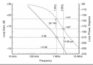
**FIGURE 4.4** Plot showing phase margin and gain margin.
