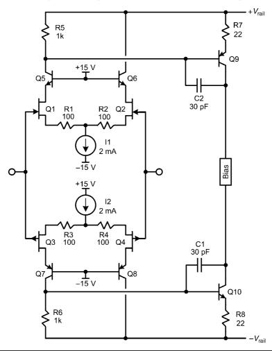
FIGURE 7.11 Complementary differential input stage with JFETs.
