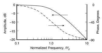
FIGURE 4.3 Gain and phase for a pole at frequencies far from the pole frequency.
