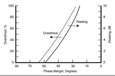
**Figure 4.10** (a) Square-wave overshoot. (b) Frequency response peaking as a function of phase margin.
