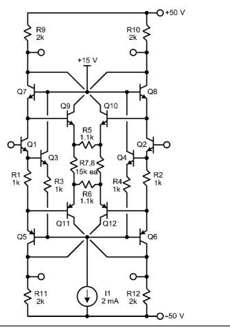
FIGURE 25.12 Complementary Cascomp input stage.
