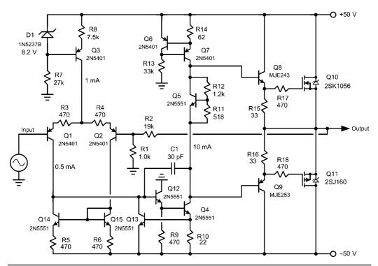
FIGURE 11.1 A simple lateral MOSFET power amplifier.
