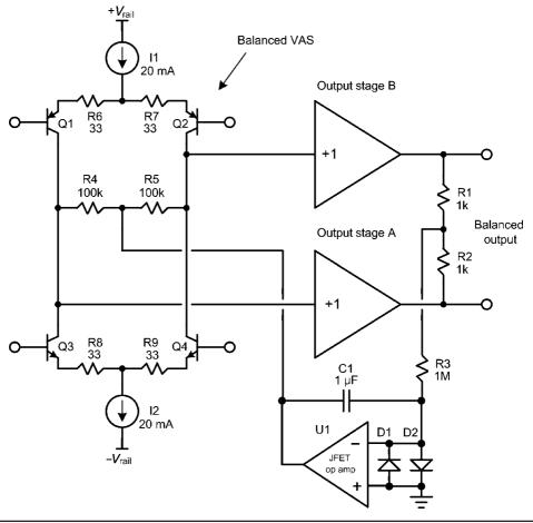
FIGURE 26.9 A common-mode DC servo arrangement.
