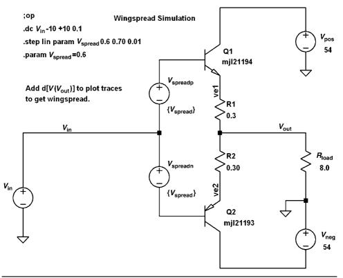
FIGURE 19.4 Wingspread simulation of a class AB output stage.
