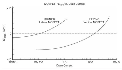
**FIGURE 14.14** Temperature coefficient of  $V_{gs}$  versus drain current for typical lateral and vertical MOSFETs.
