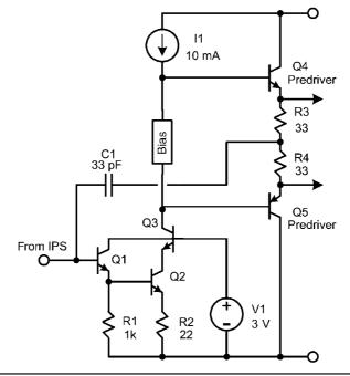
FIGURE 4.11 Example of a "longer" Miller compensation loop.
