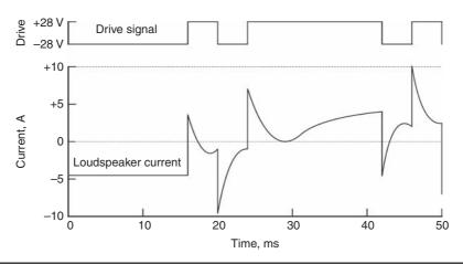
FIGURE 18.3 High peak load currents when the loudspeaker is driven with a contrived waveform.
