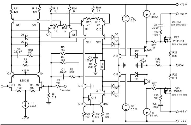
FIGURE 25.15 A MOSFET feedback amplifier with 40-kHz open-loop bandwidth.
