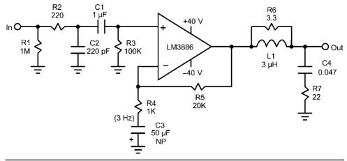
FIGURE 27.1 A 50-W Gain Clone amplifier based on the LM3886.
