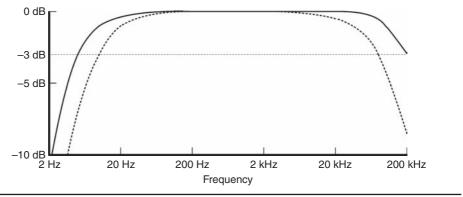
FIGURE 1.2 Amplifier frequency response.
