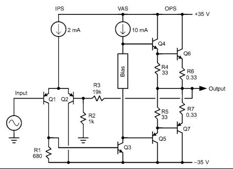
FIGURE 1.5 Simple three-stage power amplifier.
