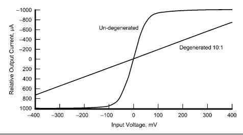
FIGURE 3.3 Differential stage current versus input voltage.
