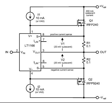
FIGURE 27.8 A simplified MOSFET output stage using the LT1166.
