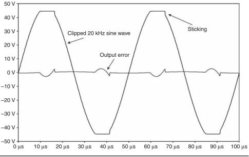
FIGURE 17.1 Output waveform of an amplifier that is clipping and sticking.
