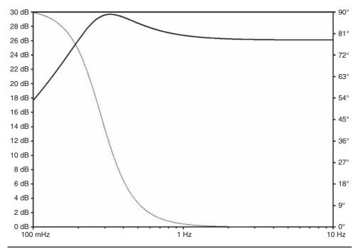
FIGURE 8.9 Frequency response of a poorly designed DC servo.
