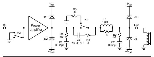
FIGURE 15.19 Some relay contact protection approaches.
