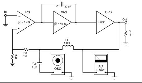
FIGURE 4.7 Breaking the loop with a large inductor.
