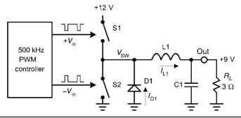
FIGURE 28.4 A synchronous Buck converter.
