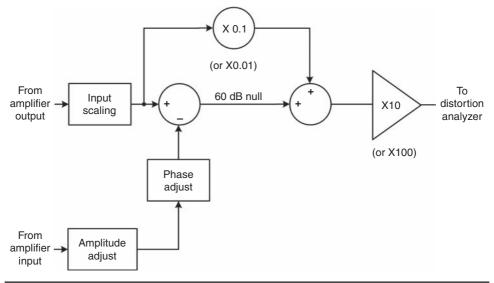
FIGURE 21.4 The Distortion Magnifier.
