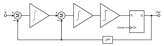
FIGURE 30.6 A second-order sigma-delta modulator.
