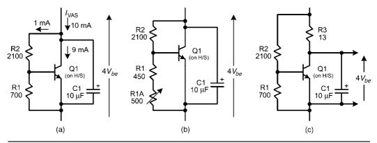
**FIGURE 14.9** Conventional  $V_{be}$  multiplier bias spreader.
