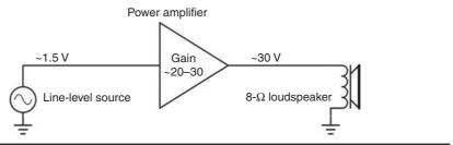
FIGURE 1.1 Power amplifier driving a load.
