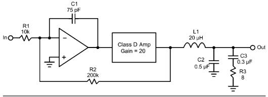
FIGURE 30.1 PWM amplifier with prefilter feedback.
