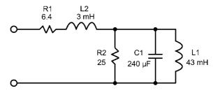
FIGURE 22.5 Loudspeaker model for simulation of peak current flow.
