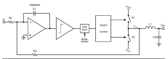
FIGURE 30.4 A self-oscillating PWM modulator employing a one-shot.
