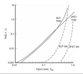
FIGURE 7.5 THD-1 for the input stages of Figure 7.4.
