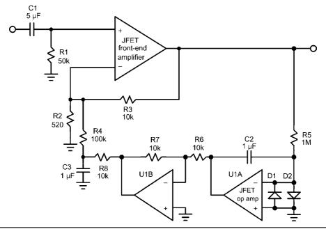
FIGURE 8.7 DC servo with additional low-pass filter.
