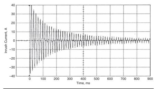
FIGURE 16.12 AC inrush current waveform for the power supply of Figure 16.1.
