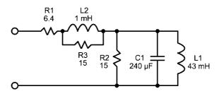
FIGURE 18.1 Electrical model of a loudspeaker woofer.
