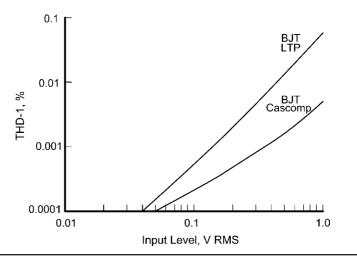
FIGURE 25.11 Cascomp THD versus differential pair THD.
