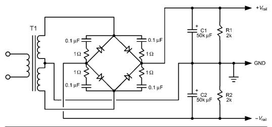
FIGURE 16.9 A bridge rectifier with snubber networks.
