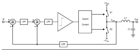
FIGURE 30.2 Self-oscillating PWM class D amplifier.
