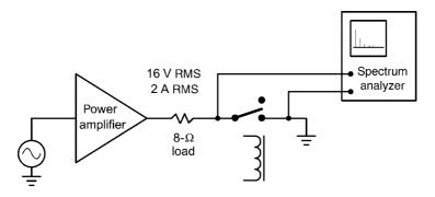
FIGURE 13.5 Test setup for measuring relay distortion.
