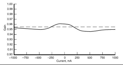
FIGURE 2.18 Output stage gain versus output current.
