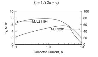
**FIGURE 20.5** Transistor  $f_{\tau}$  as a function of collector current.
