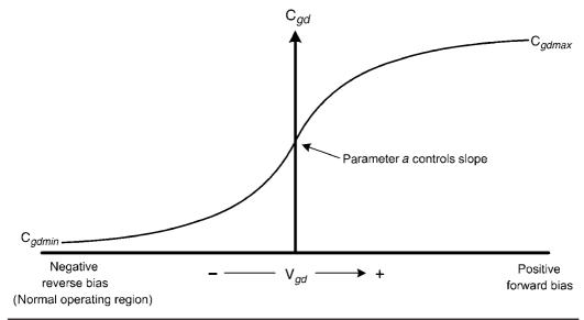
**FIGURE 20.13**  $C_{ad}$  as a function of  $V_{ad}$  in the VDMOS model, for  $V_{ad}$  large negative to large positive.
