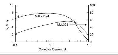
**FIGURE 10.11** Power transistor  $f_{\tau}$  versus collector current.
