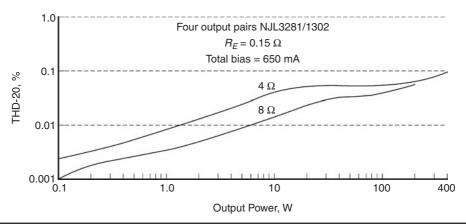
**FIGURE 25.6** THD-20 versus level for a 200-W BJT output stage. (a) Driving 8  $\Omega$ . (b) Driving 4  $\Omega$ .
