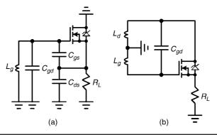
FIGURE 11.6 (a) Colpitts and (b) Hartley oscillator topologies.
