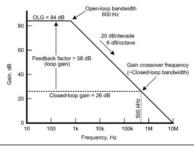
FIGURE 9.2 Bode diagram for the amplifier of Figure 9.1.
