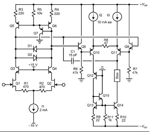
FIGURE 7.15 Differential pair VAS with current mirror load.
