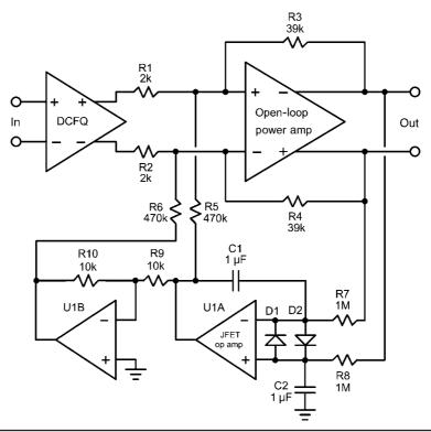
FIGURE 26.8 A balanced amplifier with differential-mode DC servo.
