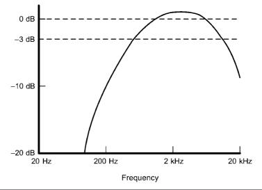
**FIGURE 7.18** A-weighting frequency response.
