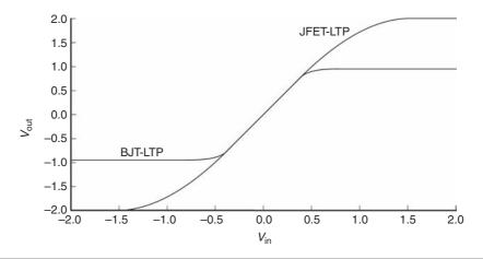
**FIGURE 7.4** Transfer characteristics for BJT and JFET differential pairs with the same transconductance.
