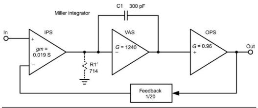
FIGURE 2.14 Amplifier gain at high frequencies.
