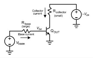
FIGURE 20.7 A measurement setup for gathering Gummel plot data.
