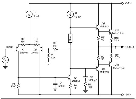
FIGURE 4.5 An amplifier where lag compensation is employed.
