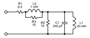
FIGURE 21.1 A passive simulated loudspeaker load.
