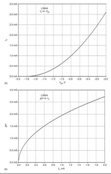
FIGURE 7.6 (a) JFET drain current as a function of gate voltage. (b) Transconductance as a function of drain current.
