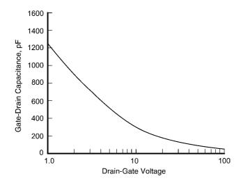
**FIGURE 11.13**  $C_{gd}$  versus  $V_{ds}$  for IRFP240.
