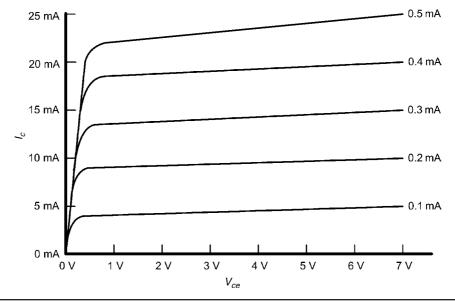
FIGURE 20.8 Transistor collector current characteristic.
