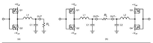
FIGURE 28.7 Half bridge and full bridge class D output stages.
