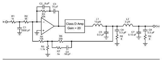
**FIGURE 29.6** An arrangement where negative feedback is taken after the primary part of the output filter.
