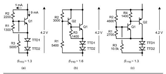
FIGURE 14.19 Bias spreaders with selectable temperature compensation.
