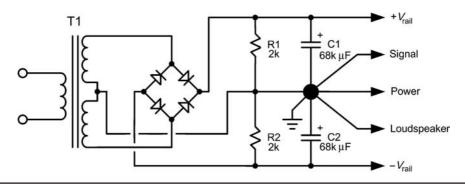
FIGURE 16.1 A typical amplifier power supply.
