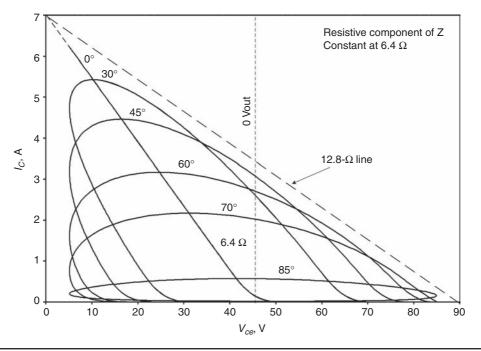
**Figure 15.7** Overlapped elliptical load lines with  $\phi = 0^{\circ}$ , 30°, 45°, 60°, and 85° when  $R_{e}$  is always 6.4  $\Omega$ .
