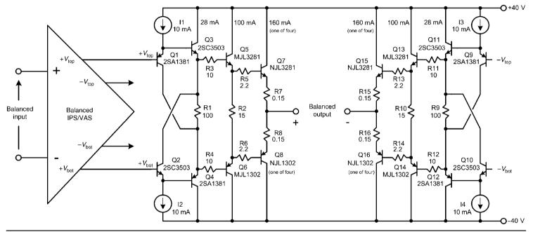
FIGURE 25.14 A 200-W balanced amplifier without negative feedback.
