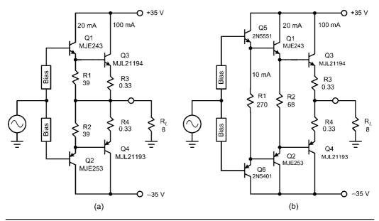
FIGURE 5.1 (a) Darlington and (b) Triple class AB output stages.
