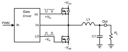
FIGURE 28.8 Half bridge output stage with N-channel high side and low side MOSFETs.
