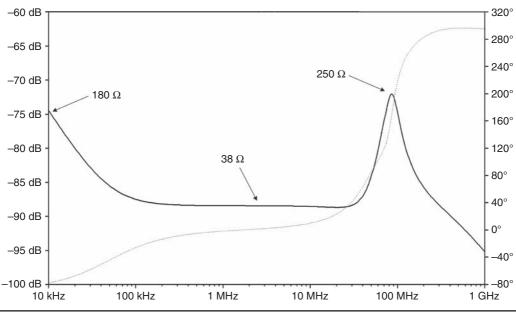
FIGURE 4.12 Stability probe result at the collector of the VAS.
