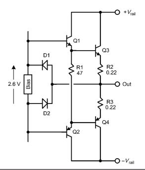
FIGURE 15.11 Natural current limiting with flying catch diodes.
