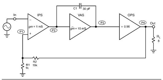
FIGURE 4.9 Probing points for stability evaluation.
