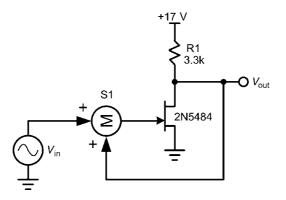
FIGURE 24.2 One-stage circuit for evaluating spectral growth distortion.
