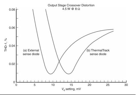
**FIGURE 14.24** Output stage crossover distortion as a function of initial bias setting V<sub>a</sub>.
