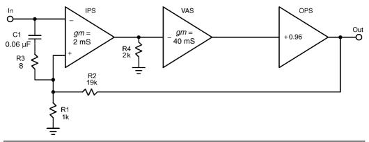
FIGURE 9.6 Amplifier with input compensation.
