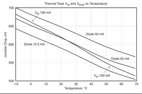
FIGURE 14.20 V<sub>ho</sub> and tracking diode drop versus temperature for different tracking diode current.
