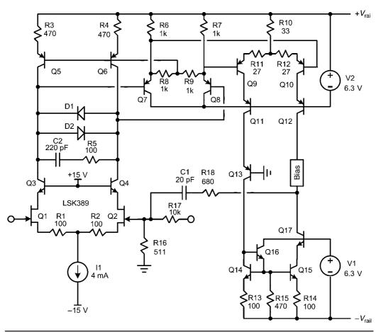
FIGURE 7.16 Input stage with differential current mirror load.
