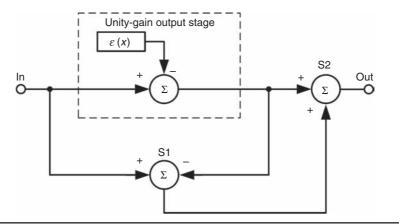
FIGURE 12.1 Feed-forward error correction.
