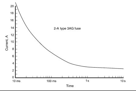
FIGURE 15.9 Typical fuse characteristic for a 2-A type 3AG fuse.
