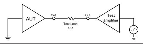
FIGURE 15.17 Back driving an amplifier to test SOA protection.
