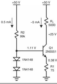
FIGURE 2.10b Current source using diodes.
