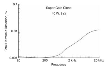
FIGURE 27.4 THD versus frequency at full power (40 W).
