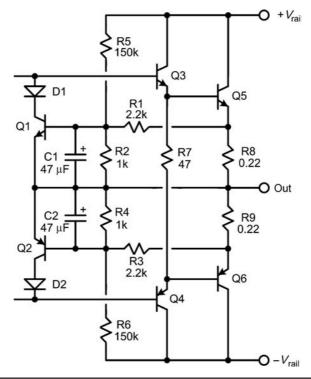
FIGURE 15.14 A single-slope V-I limiter.
