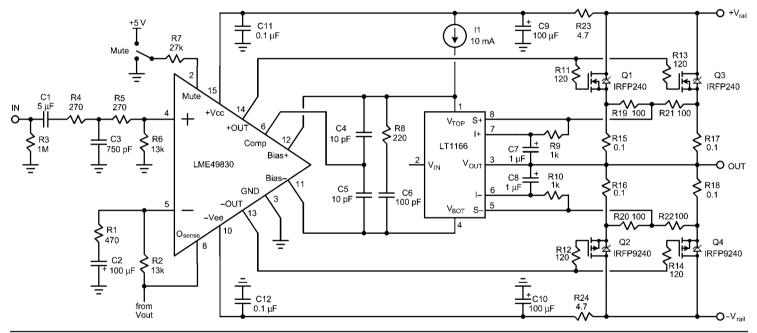
FIGURE **27.10** A MOSFET power amplifier based on the LT1166 and LME49830.
