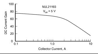
FIGURE 10.16 Beta versus I<sub>c</sub> for the MJL21193.
