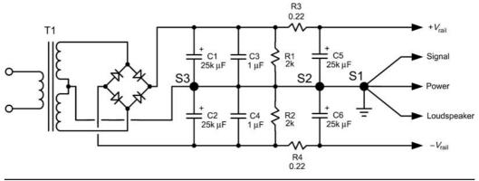
FIGURE 16.8 Split reservoir capacitor arrangement.
