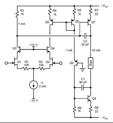
FIGURE 7.14 N-channel input stage with complementary VAS.
