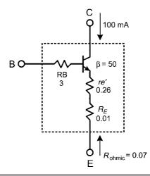
FIGURE 10.8 Dynamic emitter resistance components.
