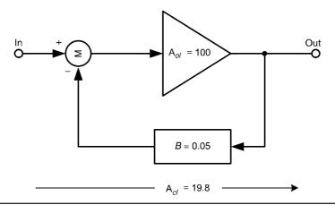
FIGURE 4.1 Block diagram of a negative feedback amplifier.
