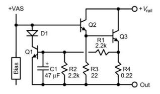
FIGURE 15.10 Simple current-limiting circuit.
