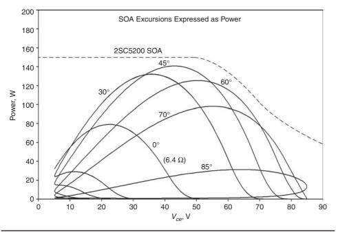
FIGURE 15.8 SOA and transistor stress plotted in terms of power.
