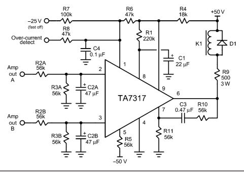
FIGURE 15.18 Typical protection circuit using the TA7317.
