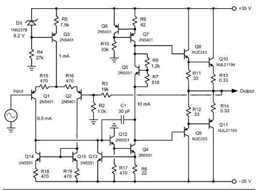
FIGURE 3.8 Input stage with current mirror load.
