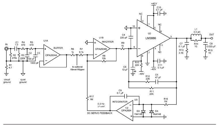
FIGURE 27.3 The Super Gain Clone employing a DC servo.
