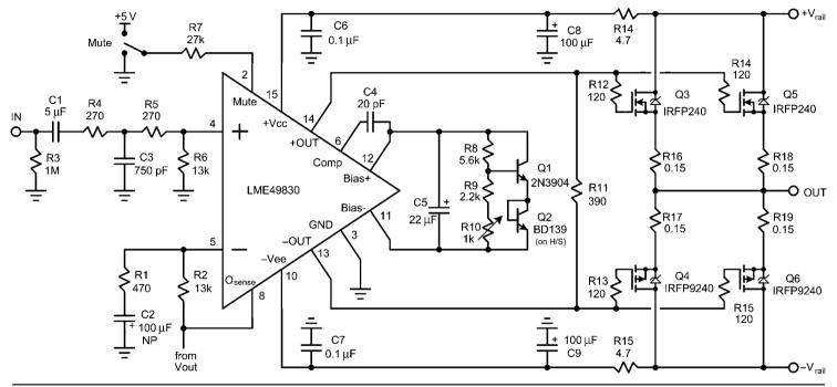
FIGURE 27.7 A MOSFET power amplifier based on the LME49830.
