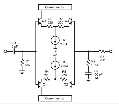
FIGURE 8.4 The complementary input differential pair.
