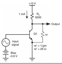
FIGURE 2.5a Common-emitter amplifier.
