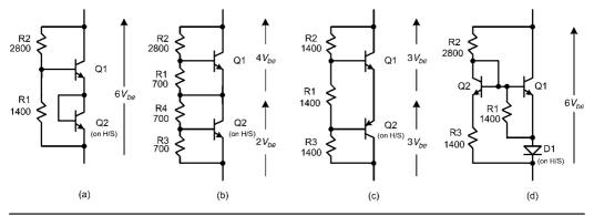
FIGURE 14.11 Four different split bias spreader arrangements.
