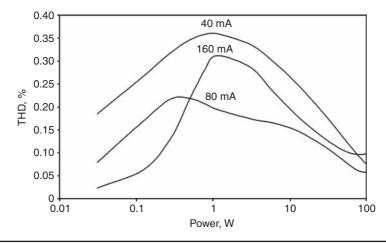
FIGURE 10.3 Crossover distortion versus power level.
