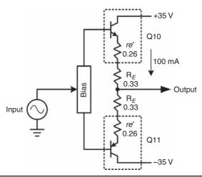
FIGURE 2.16 Push-pull output stage.
