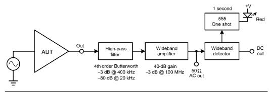
FIGURE 23.2 Block diagram of a parasitic oscillation sniffer.
