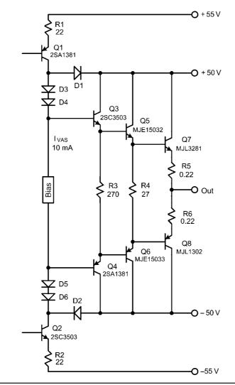
FIGURE 17.2 A simple power amplifier with a Baker clamp.
