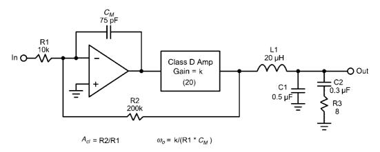
FIGURE 29.5 PWM amplifier with negative feedback taken before the filter.
