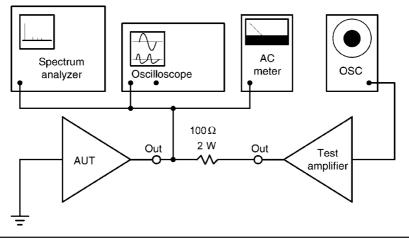
FIGURE 23.1 Measurement of damping factor.
