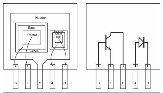
FIGURE 14.17 ThermalTrak<sup>™</sup> output transistor illustration.
