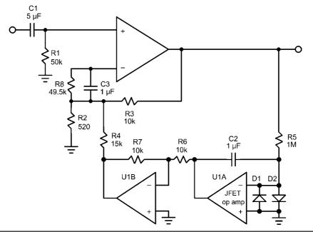
**FIGURE 8.10** Example power amplifier with a DC servo.
