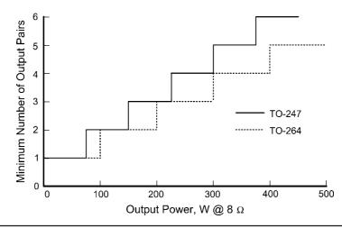
FIGURE 14.8 Recommended number of output transistors versus rated power into 8  $\Omega$ .
