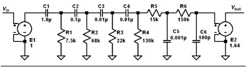
FIGURE 19.2 A-weighting noise filter.
