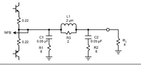
FIGURE 10.13 An output network arrangement.
