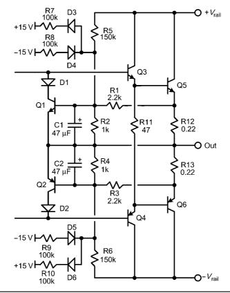
FIGURE 15.16 Three-slope V-I limiter.
