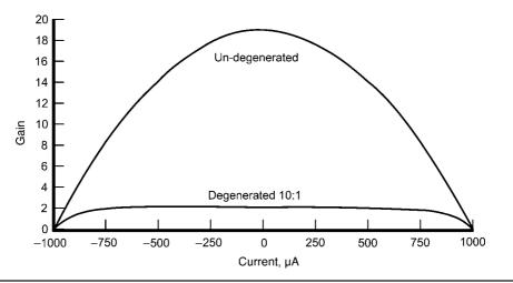
FIGURE 3.4 Differential stage gain versus output current.
