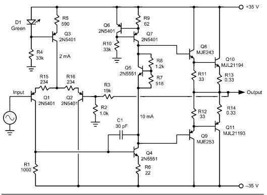
FIGURE 3.2 Input stage emitter degeneration.
