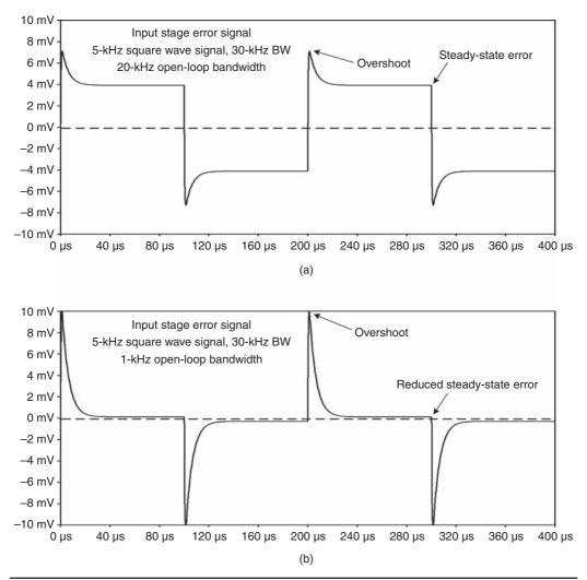
FIGURE 24.1 Input stage error signal. (a) With wide open-loop bandwidth, (b) With low open-loop bandwidth.
