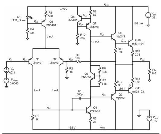
FIGURE 19.7 Power amplifier to be simulated.
