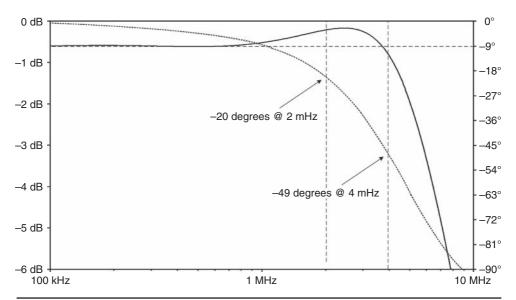
**FIGURE 10.14** Gain and phase of the output Triple driving a 4- $\Omega$  load and 0.01  $\mu$ F.
