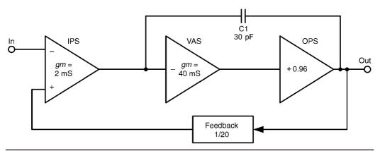
FIGURE 9.8 Amplifier with inclusive Miller compensation.
