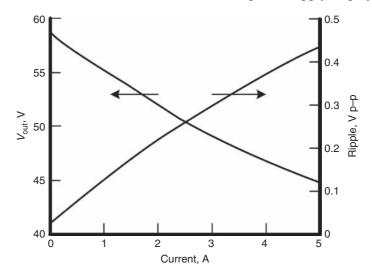
**FIGURE 16.3** Output voltage as a function of load current;  $R_{off} = 2.6 \Omega$ .
