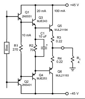
FIGURE 10.12 A Triple with a speedup capacitor.
