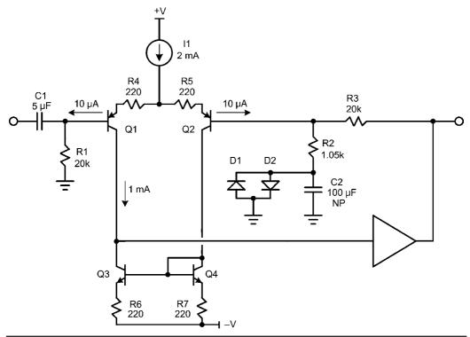
FIGURE 8.1 Conventional amplifier DC block arrangement.
