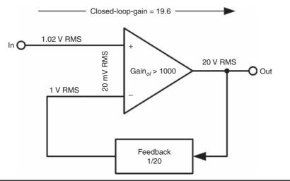
FIGURE 1.6 Negative feedback operation.
