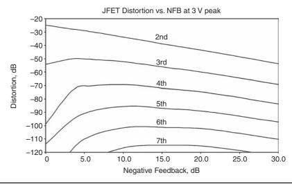
FIGURE 24.3 Harmonic distortion components versus amount of negative feedback.
