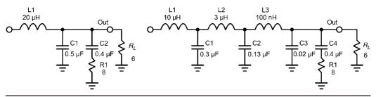
FIGURE 29.1 Example of second- and fourth-order output filters with Zobel networks.
