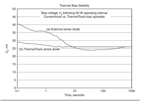
**FIGURE 14.23** Bias  $(V_c)$  as a function of time after a thermal step.
