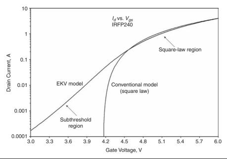
**FIGURE 20.16** MOSFET  $I_d$  versus  $V_{qs}$  for conventional and EKV SPICE models.
