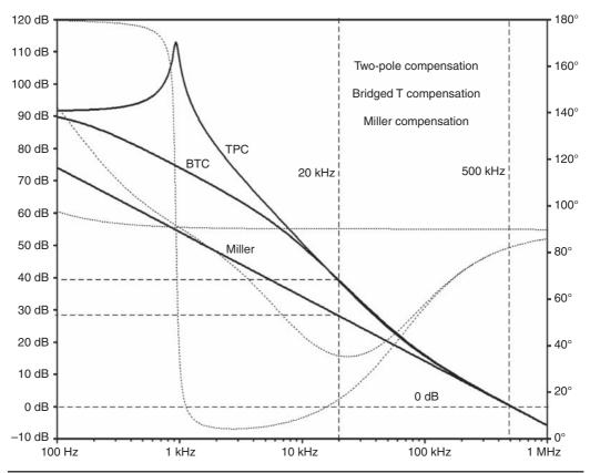
FIGURE 9.5 Loop gain plots for amplifiers with two-pole compensation and bridged T compensation.
