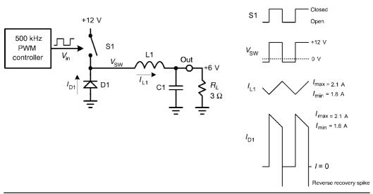
FIGURE 28.3 A Buck converter switching supply.
