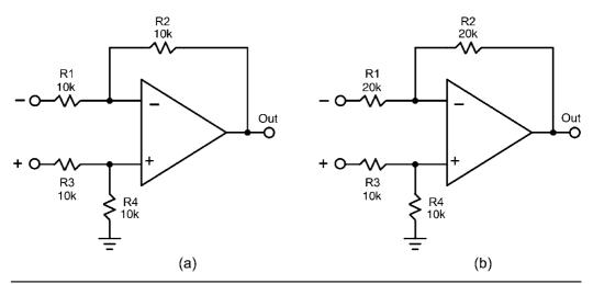
FIGURE 26.1 Single op-amp differential-to-single-ended input circuits.
