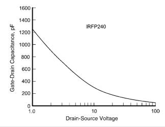
**FIGURE 20.11** Power MOSFET  $C_{ed}$  versus  $V_{ds}$  for IRFP240.
