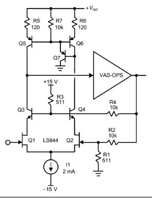
FIGURE 7.17 N-channel input stage with driven cascode.
