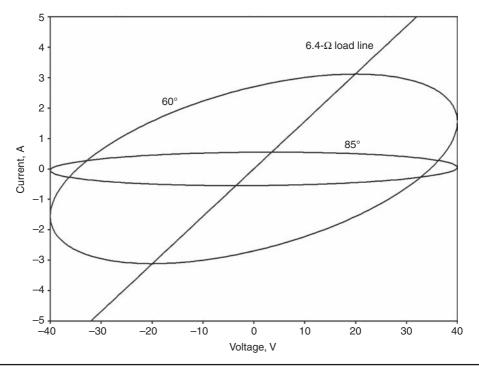
**FIGURE 15.6** Load impedance curves for  $|\phi| = 0^\circ$ , 60°, and 85° when  $R_a$  is held constant at 6.4  $\Omega$ .
