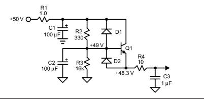
FIGURE 16.11 A capacitance multiplier filter.
