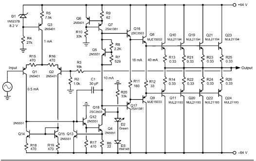
FIGURE 3.14 High-power version of the amplifier.
