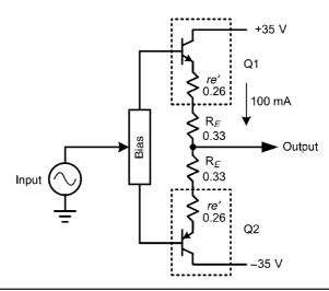
FIGURE 5.2 Output stage impedance.
