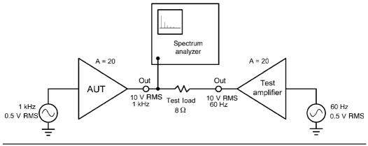
FIGURE 22.7 Measurement setup for interface intermodulation distortion.
