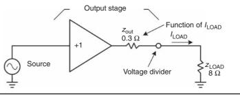
FIGURE 2.17 Amplifier output stage gain.
