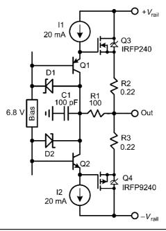
FIGURE 11.16 A MOSFET output stage with folded drivers.
