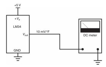
FIGURE 14.7 Using an LM34 to make temperature measurements.
