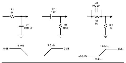
FIGURE 4.2 R-C circuits implementing poles and zeros.
