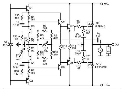
FIGURE 12.7 Breaking the loop for stability analysis.
