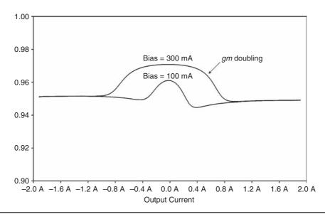
FIGURE 5.5 The gm-doubling effect in an overbiased class AB output stage.
