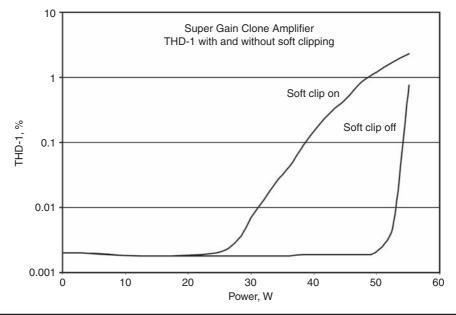
FIGURE 17.5 THD-1 versus power for an amplifier using the Klever Klipper.
