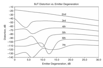
FIGURE 24.4 Harmonic distortion components versus amount of emitter degeneration NFB.
