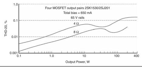
FIGURE 25.8 THD-20 versus level for a 200-W MOSFET output stage. (a) Driving 8  $\Omega$ . (b) Driving 4  $\Omega$ .
