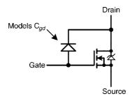
FIGURE 20.12 Subcircuit model schematic.
