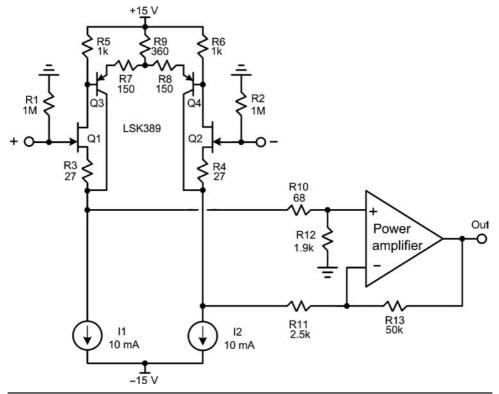
FIGURE 26.5 The differential complementary feedback Quad (DCFQ) buffer.
