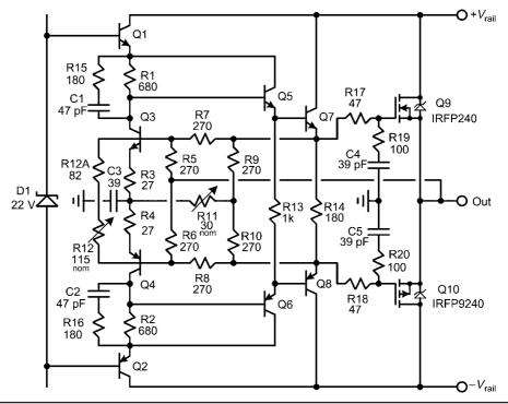
FIGURE **12.6** The error-correction circuit used in Ref. 2.
