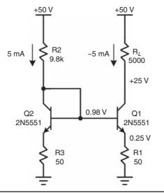
FIGURE 2.10e Current mirror current source.
