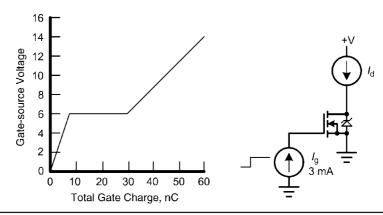
FIGURE 28.6 (a) Gate charge diagram. (b) Measurement setup.
