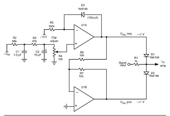
FIGURE 17.4 The Klever Klipper soft-clip circuit.
