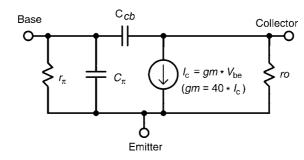
FIGURE 20.2 Hybrid pi model of a BJT.
