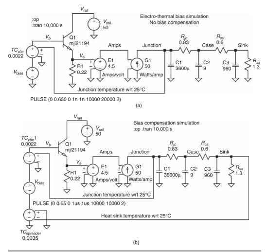
**Figure 14.6** (a) Electrothermal simulation of a transistor mounted on a heat sink. (b) Transistor's bias is controlled by a  $V_{he}$  multiplier.
