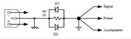
FIGURE 16.14 Breaking a safety ground loop.
