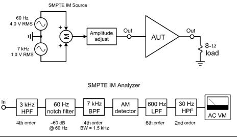
FIGURE 22.1 Measuring SMPTE intermodulation distortion.
