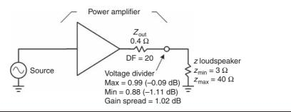
FIGURE 1.4 Amplifier output impedance.
