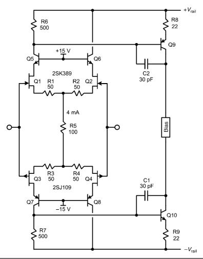
FIGURE 7.12 Complementary differential input stage with floating JFETs.
