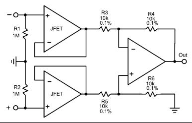
FIGURE 26.2 Triple op-amp instrumentation amplifier.
