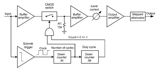
FIGURE 21.5 A synchronous tone-burst generator.
