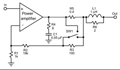
FIGURE 17.6 Selection of amplifier output impedance.
